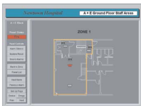
Highest zoom showing detector in alarm
